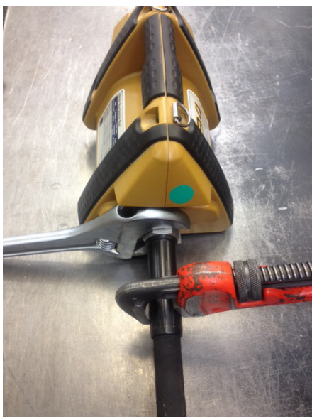
Figure 10: Crescent wrench and pipe wrench placement
